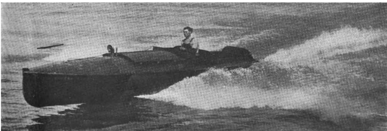
Sutter Basin, a Pacific Coast Monoplane. Power 6-Cylinder 5½ In. x 6 In. 45-75-H.P. Sterling Engine. Speed 31 Miles per Hour. Mr Silva Owner
